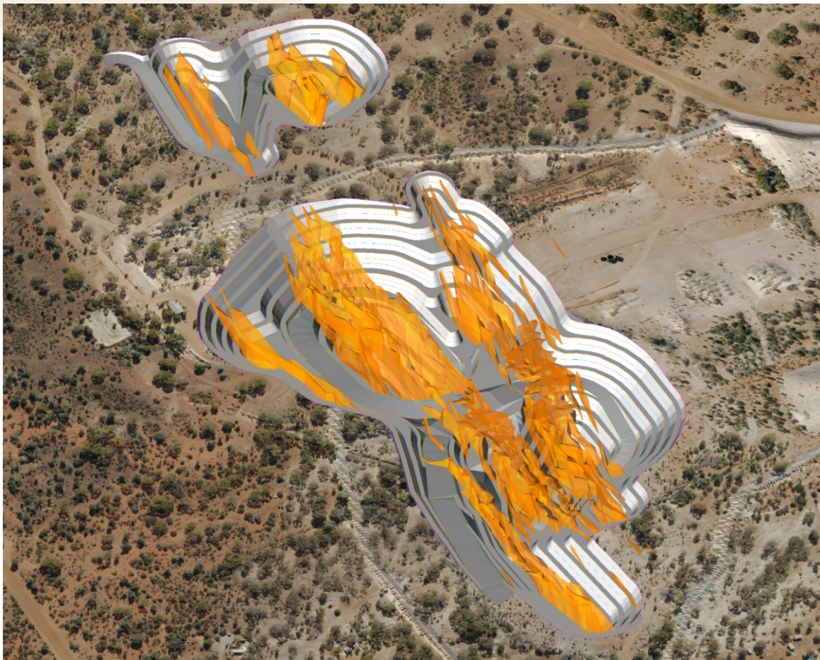
Figure 4 - Riverina open pit design showing mineralised lodes
